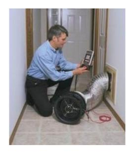
Any duct systems located totally or partially outside the conditioned space, such as supplies or returns in attics or crawlspaces, behind knee walls, or other unconditioned spaces, MUST be tested.
